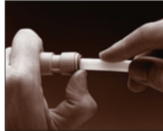
3. To disconnect push in collet and pull tubing
